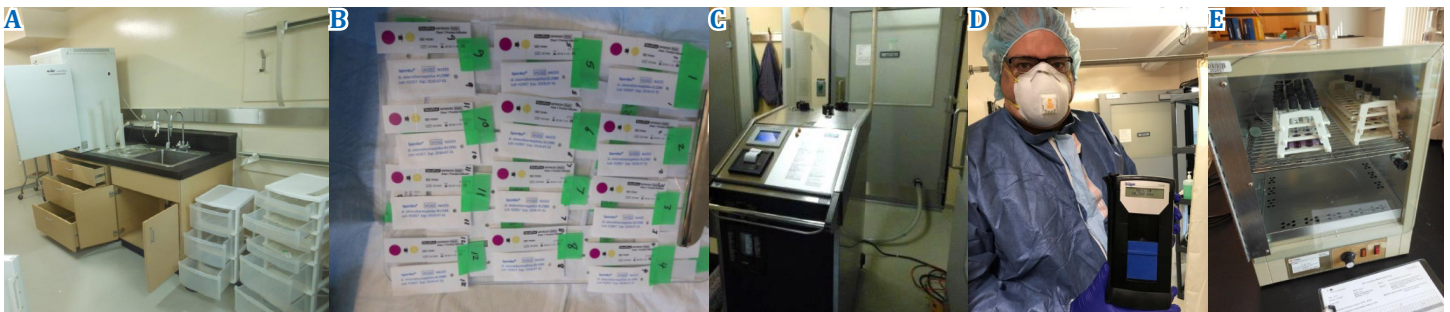
Figure 2. Components of the decontamination process including A: surface cleaning/disinfection and preparation, B: biological and chemical indicator preparation, C: preparation/installation of the gas sterilization system, D: Biosafety Officer John Tansey tests hydrogen peroxide levels post decontamination, E: incubation of biological indicators to determine success of the procedure.
