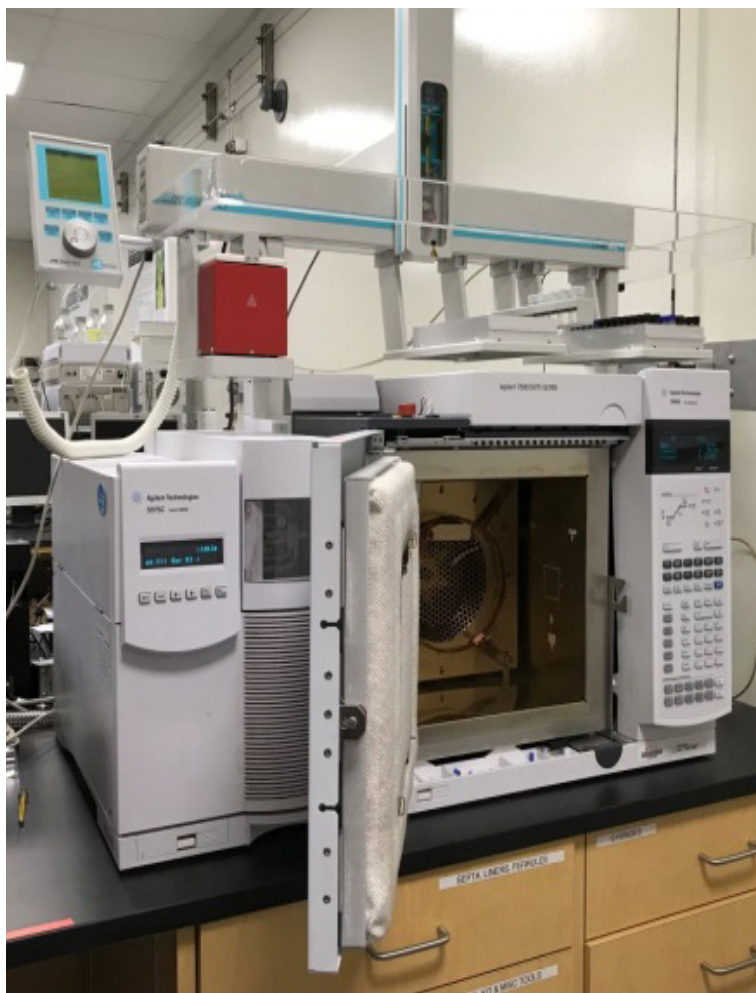
Figure 7. Headspace GC/MS instrument at BCIT used to measure ethanol levels in kombucha samples
