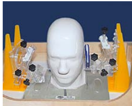
Figure 4.4 Example of a head phantom assembly for inner probe measurements 6
