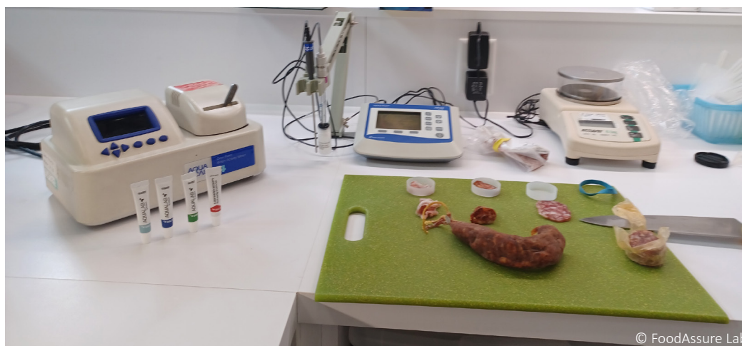
Figure 3 | Water activity ( a_w ) testing of sausage samples
