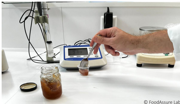
Figure 2 | pH equipment being used to test acidity of jam
