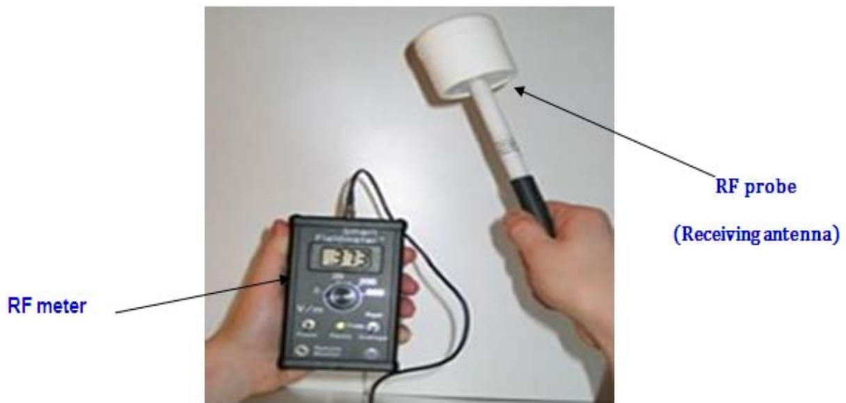
Figure 4.2 Portable RF survey meter
