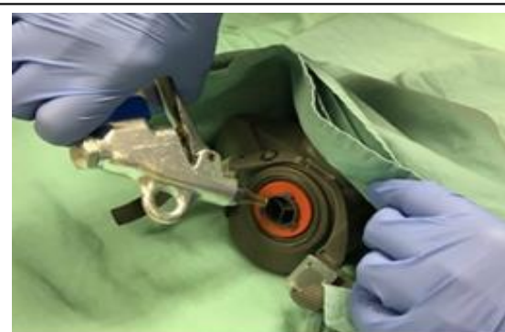
Figure 2: Use of regulated compressed air to dry excess moisture from respirator.
